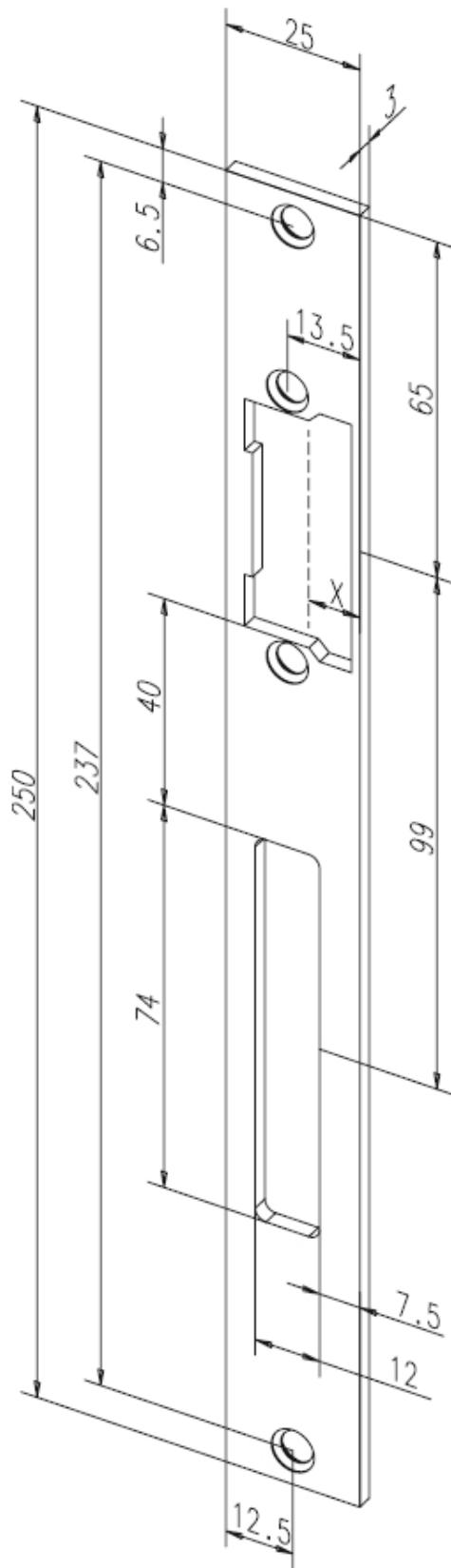
ProFix 2 flat striking plate with latch bolt aperture and dead bolt cutout.
