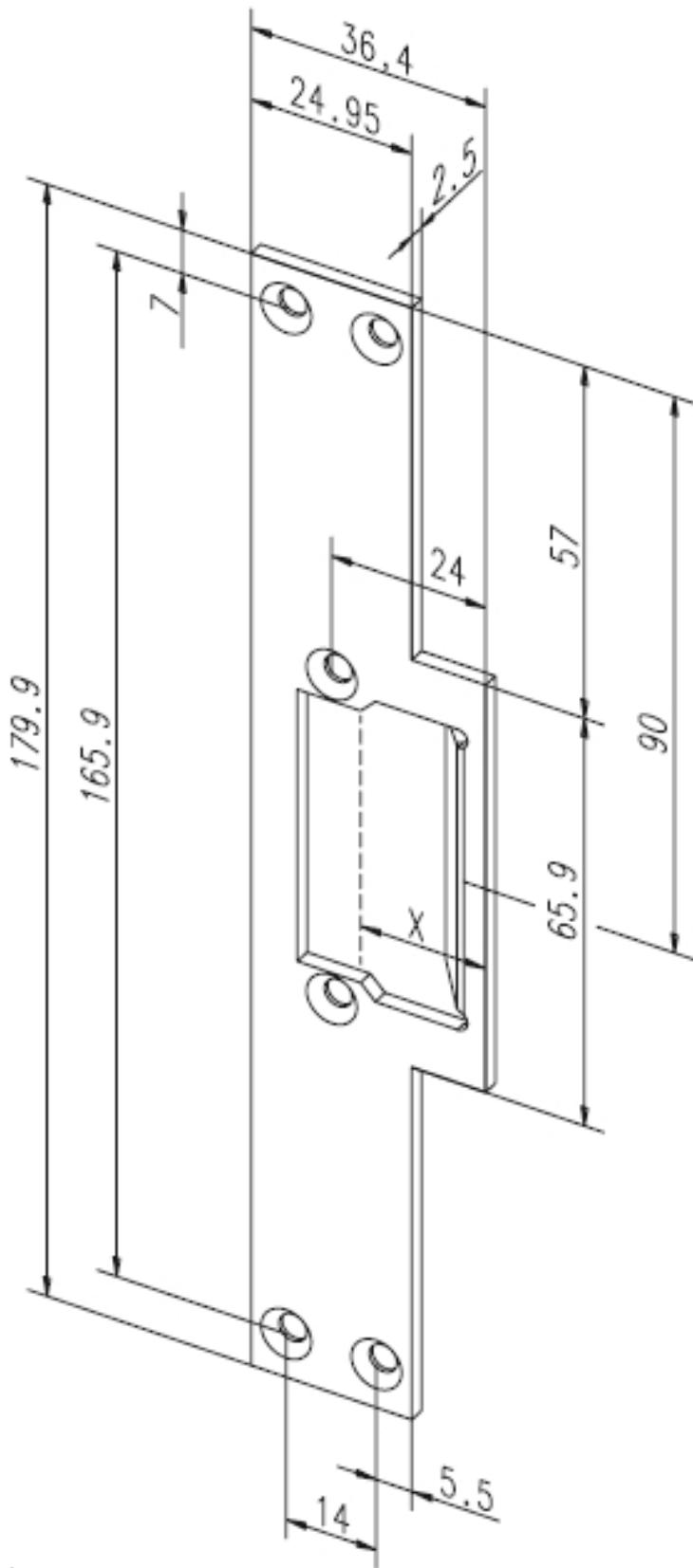
Short flat striking plate with latch bolt aperture.
